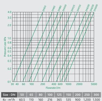
The maximum recommended flow velocity inside the pipe is 1.2 m/s. The following shows the maximum flow rates to meet this requirement.
